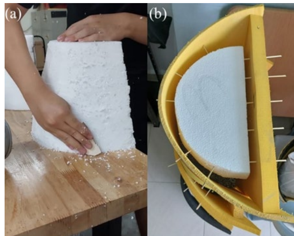
Figure 4. (a) Crafting stacked polystyrene for water retaining feature and (b) basin mould created with thick modelling foam (Source: Authors)
