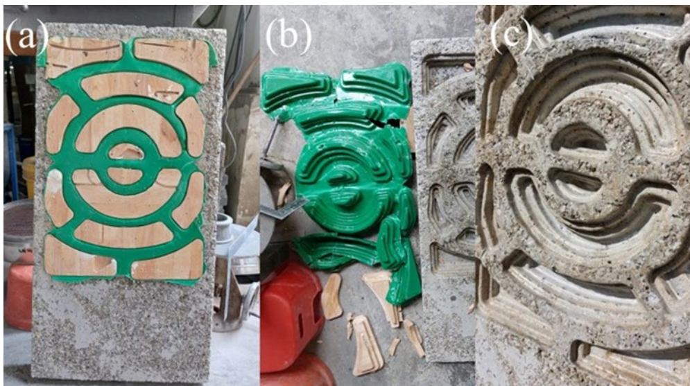
Figure 9. (a) Vacuum formed mould stuck to model, (b) removal of vacuum formed mould via destruction, and (c) smooth surfaced appearance of the model's designs (Source: Authors)
