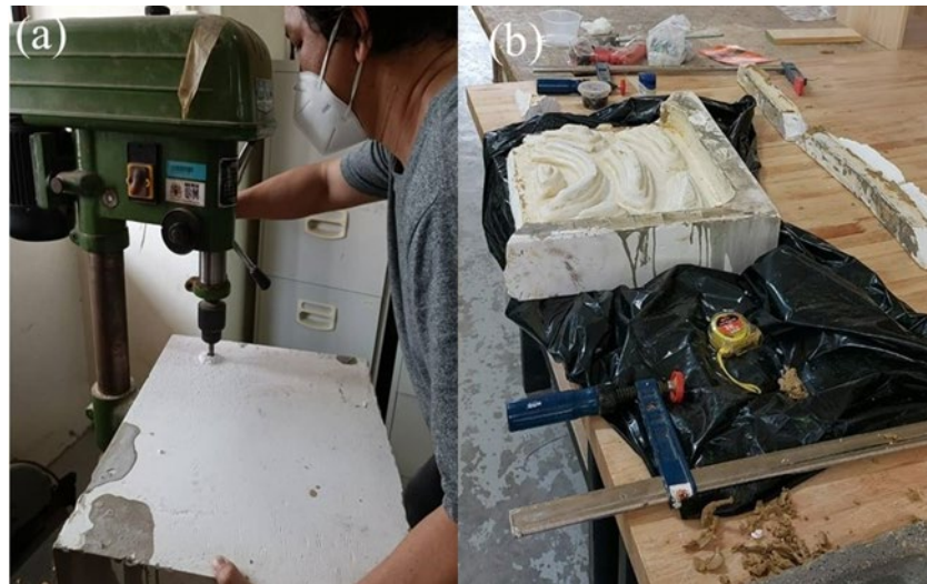
Figure 6. (a) Drilling holes onto corners of the plaster mould for compressed air to push through casted concrete and (b) broken sides of plaster mould which was held together by clay, hot glue, and clamps for next casting (Source: Authors)
