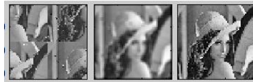
Fig. 5 (Left) The 8-bit gray scale watermark w'(p,q) extracted with some error pixels; (Middle) The error-reduced w''(p,q) produced from remapping w'(p,q) and smoothing; (Right) The down-scaled version of the test image for authentication.
