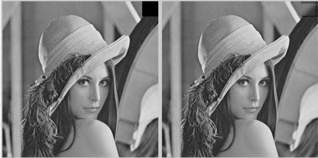
Fig. 7 (Left) Top-left corner cropping on the stego image (Right) Approximately recovered content without edge details.
