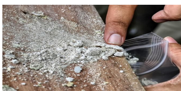
Figure 18: Collect Specific Amount of Sample and Put in the Zip Bag with Tagging
