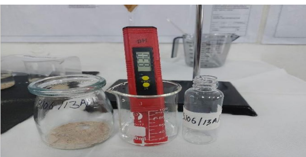
Figure 35: Check the Ph Level Before Place the Solution in the Clean Bottle
