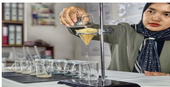
Figure 32: Filter the Solution to Remove any Undissolved Particles
