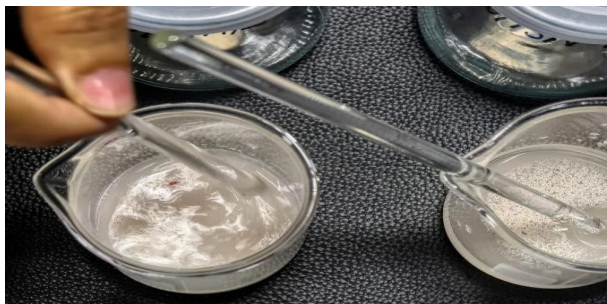
Figure 31: Stir the Sample in the Beaker with Deionized Water (20 ml)
