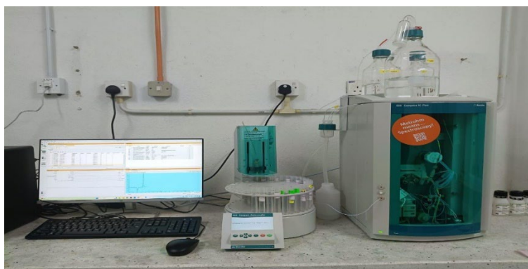
Figure 39: Setup Instrument for Ion Chromatography Testing
