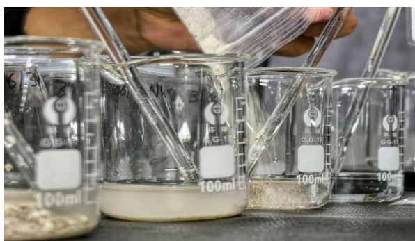
Figure 30: Sample in the Beaker with Deionized Water (20 ml)
