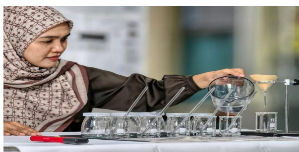
Figure 27: Place Deionized Water in the Beaker (20 ml)
