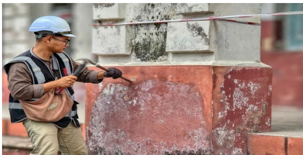
Figure 15: Crushing the Point Selected to Collect the Sample
