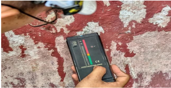
Figure 13: Measure the Moisture Content Before Pointing the Place to take the Materials
