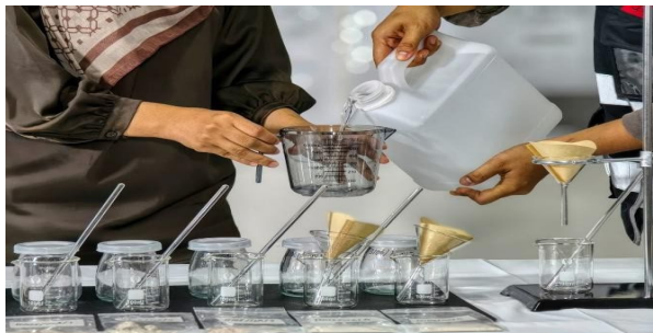
Figure 26: Place Deionized Water into Measured Jug to Easy Put in the Beaker (20 ml)
