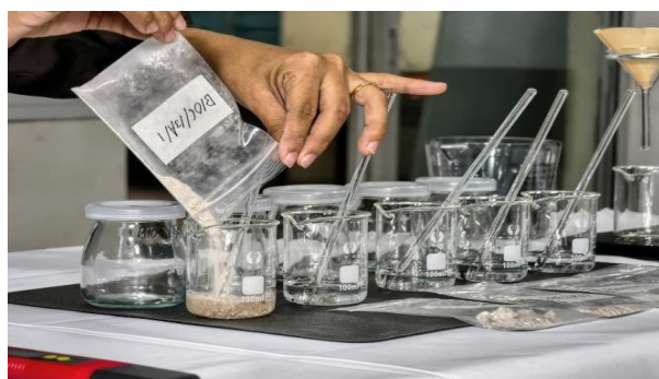
Figure 29: Place Specific Amount of the Sample in the Beaker with Deionized Water (20 ml)
