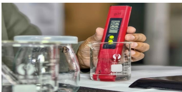
Figure 35: Check the Ph Level Before Place the Solution in the Clean Bottle
